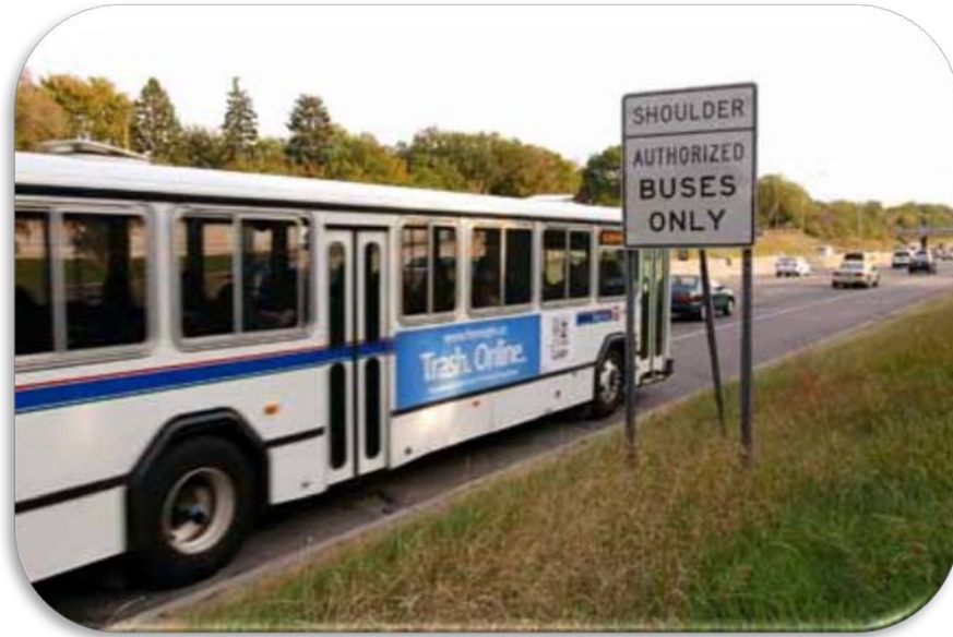
Figure 19. Photo. Mn/DOT BOS Regulatory Sign (Photo Courtesy of Mn/DOT).
